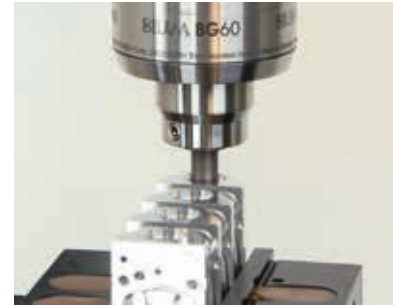
Diameter Measurement with BG60
