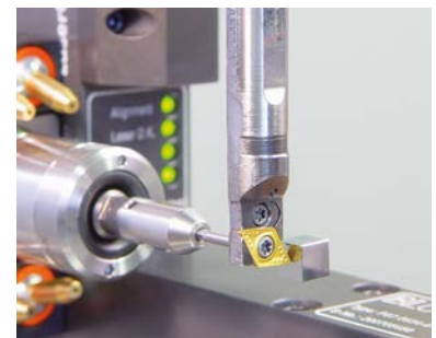
Extremely fast measurement of non-rotating tools
