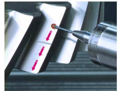
Scanning procedure for checking of workpiece surface
