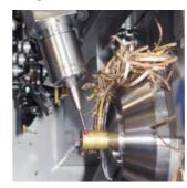
Tool measurement – TC76 with protective sleeve
