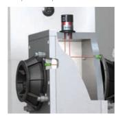
TG81: Temperature sensor and transmission unit
