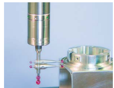
shark360 measuring mechanism enables pulling/pushing measurements in Z+/Z-
