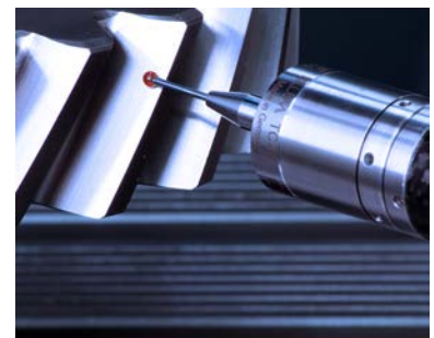
Workpiece measurement in grinding centre
